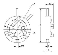
The model 830-0010 and model 830-0020 self-centring lens mounts reliably centre and safely hold round optics and cylindrical components. Holding by three rods with V-groove tips provide easy and secure optics accommodation with high relocation repeatability.
